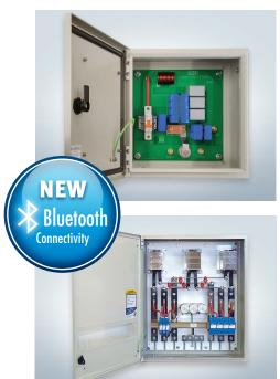
Series powerline protection is the best available protection for sensitive electronics such as rectifiers, switchmode power supplies, and other mission critical equipment. The Series Filter reduces the rate of rise of any transient overvoltage to acceptable levels, and also reduces the overall magnitude of the transient voltage the equipment receives.
